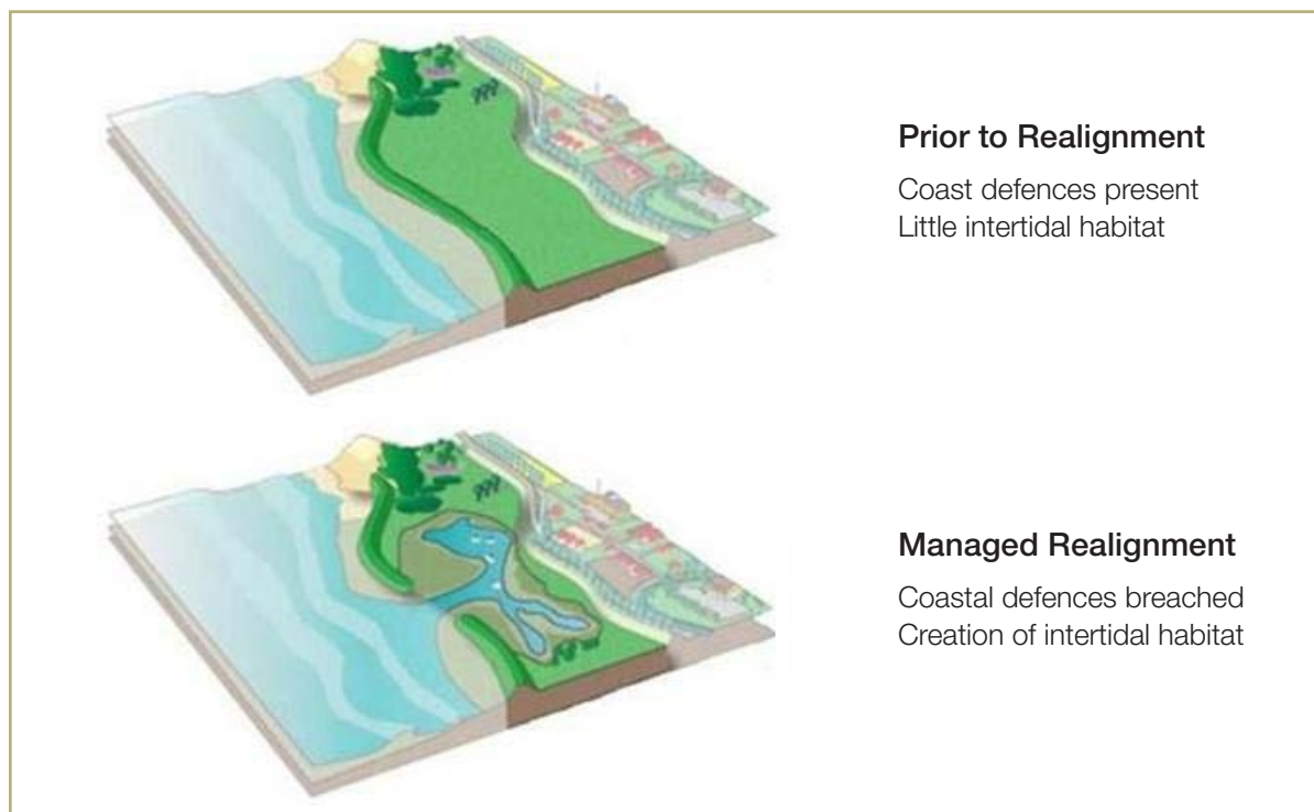
Figure 4.28: The process of managed realignment
